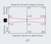
Note: The sensor will measure at longer distances than shown, with a larger measured spot diameter. Contact Calex for more information.
