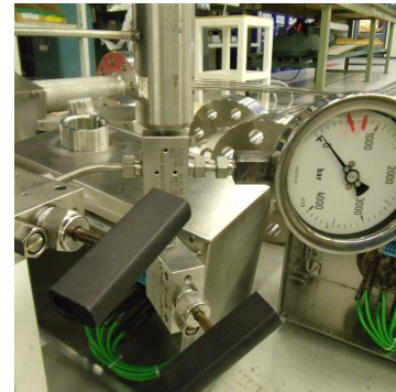
External pressure testing
