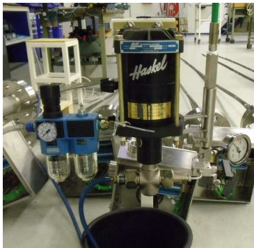
Internal pressure testing
